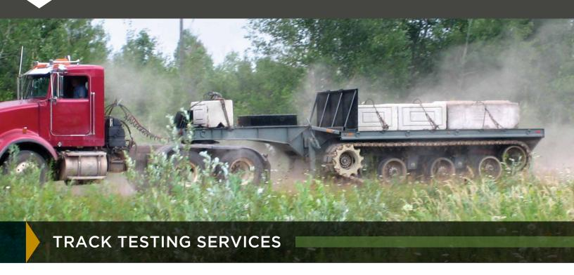
GS Engineering has developed a novel way to field test track components under SBIR A08-131. The Track Testing Trailer offers capabilities never before offered in a sub scale track testing device.
